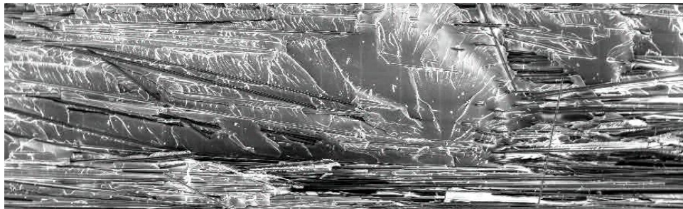
Figure 105 - Brittle fracture seen in dry specimens
