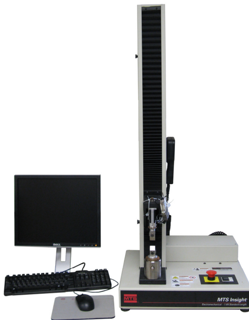
Figure 35 - MTS Insight 1kN test machine in the fiber tensile testing configuration
