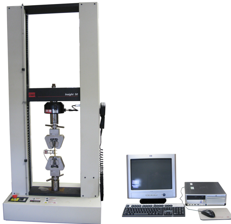
Figure 47 - MTS 50 Insight test machine configured for resin tensile-testing
