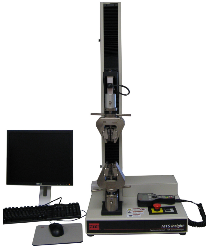
Figure 84 - MTS Insight 1kN test machine in the transverse tensile testing configuration
