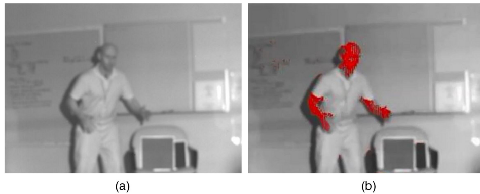
Fig. 14 Screen shot from video of dual-camera skin detection system (a) without skin detection applied and (b) with skin detection.
