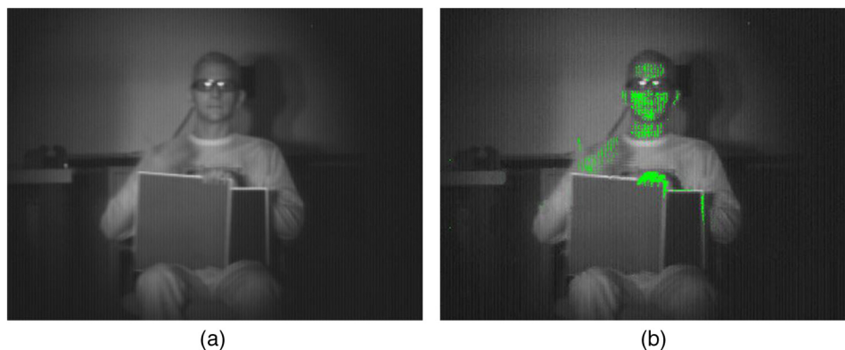
Fig. 18 Screenshot of the skin detection video processed through the wavelength-switching optical box (a) without skin detection applied and (b) with skin detection.
