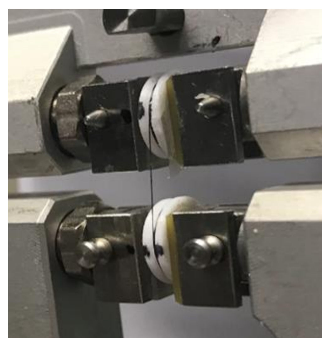
Figure 3 - Fiber being tensile tested with PMMA clamps and PLA discs.
