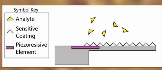
NSWC-PCD is interested in a similar application using micocantilevers which directly measure deflection via an internal piezoresistive element. A sensitive coating, such as our composite material, applied to the surface of the cantilever would induce a deflection of the beam in the presence of analytes, again due to the change in surface stress.
