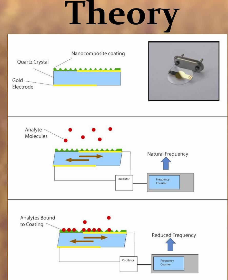
A quartz crystal microbalance (QCM) undergoes shear oscillation when activated by an AC current to it's electrodes. When coated, the frequency of this oscillation becomes a function of the surface stress generated by the adhesion of the coating to its surface. If another compound then binds to this coating, it will apply a different amount of stress to the crystal. This will in turn change the frequency in proportion to the amount of foreign material bound to the coating.
